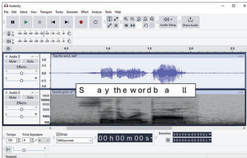
Fig. 2.8 Screenshot of the Audacity software showing a recording of the phrase "Say the word ball." We can easily see amplitude variations over time (top) and the spectrogram (below) shows spectral changes over time.
